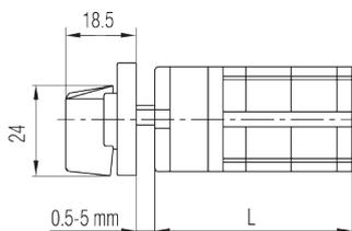
**GF20** Ugradna sklopka / *Front mounting (U)*
